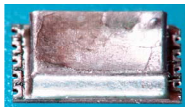
Fig. 10 Crushed TCXO
